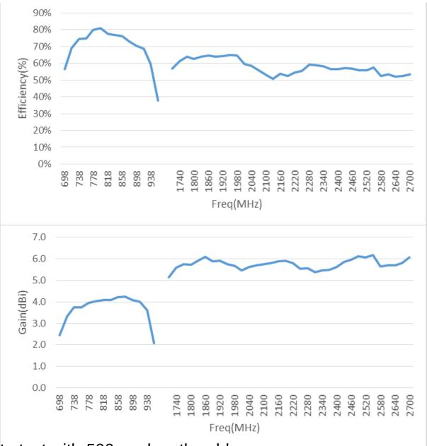
All data test with 500mm length cable
