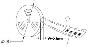
1. Material: Black Conductive Polystyrene 2. Components per Reel: see table
