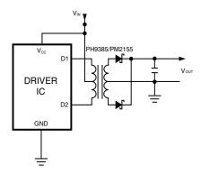
For a fixed 50% duty cycle mode of operation, the output voltage is simply determined by the input voltage and turns ratio. So, with the available turns ratios, a variety of output voltages can be selected. This range can be extended by implementing different topologies such as forward or bridge and can be used with controllers offered by different IC vendors for a number of different applications.
