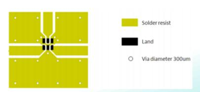
Line width should be designed to match  $50\Omega$  characteristic impedance, depending on PCB material and thickness.
