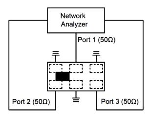
Test Instrument: Agilent E5071C Network Analyzer or equivalent.
