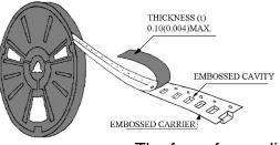
The force for peeling of cover tape is 10 grams in the arrow direction.
