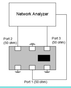
Test Instrument : Agilent E5071C Network Analyzer or equivalent.
