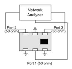
Test Instrument : Agilent E5071C Network Analyzer or equivalent.
