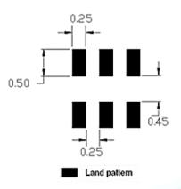
Unit : mm Line width should be designed to match  $50\Omega$  characteristic impedance, depending on PCB material and thickness.
