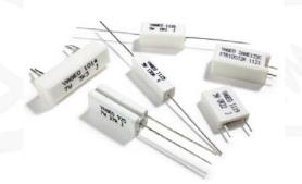
Yageo produces cement resistors in non-inductive, metal plate, fusible, wirewound, thermal, anti-explosion and anti-arc styles. Power ratings from 2W to 10W and resistance values between 0.015  $\Omega$  to 1M  $\Omega$  are available. These resistors come with axial, vertical, and radial lead types, and are all housed in a flame-proof ceramic case.
