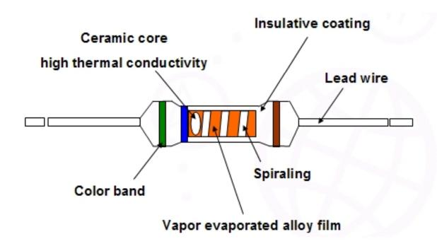
The resistance value is then achieved by cutting spirals into the vapor evaporated alloy film.
