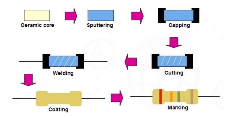
The first phase of forming a high stability, narrow tolerance leaded resistor is sputtering a layer of special resistant alloy onto a high grade ceramic.
