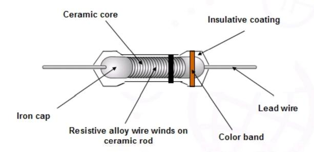
In an entirely different process from film resistors (which are cut from a ceramic core), wirewound resistors are made by winding a wire around the ceramic core. The resistance value of a leaded wirewound is determined by the number of revolutions of the alloy wire around the ceramic core.
