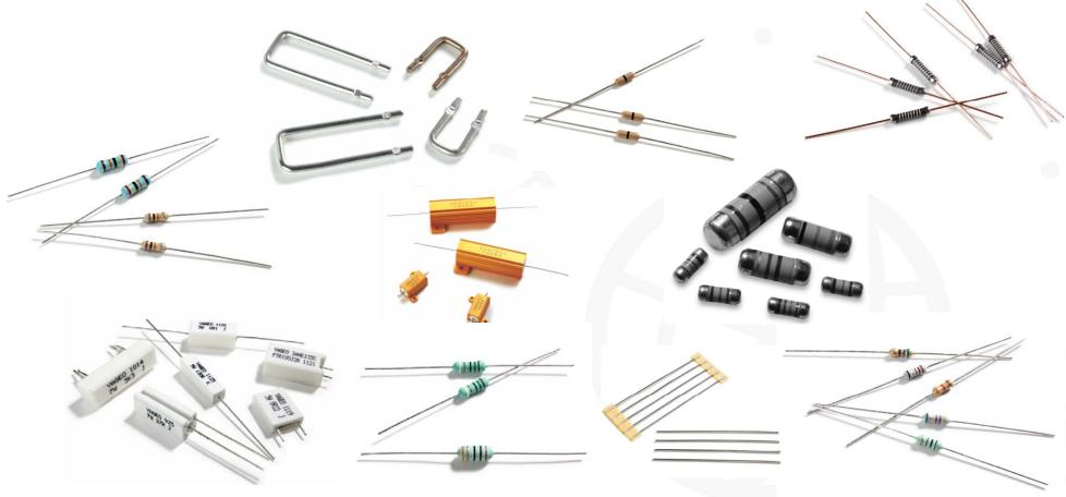
Leaded resistors are also called through-hole resistors, come in small, cylinder-like packages with axial wire leads (the wires come out the main axis of the cylinder). They are marked with either colored bands or numerically to determine their resistance. Some through-hole resistors are not cylindrical, but rectangular. These resistors are know as *power resistors* due to their ability to handle large power loads.
