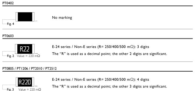
For further marking information, please refer to data sheet "Chip resistors marking".
