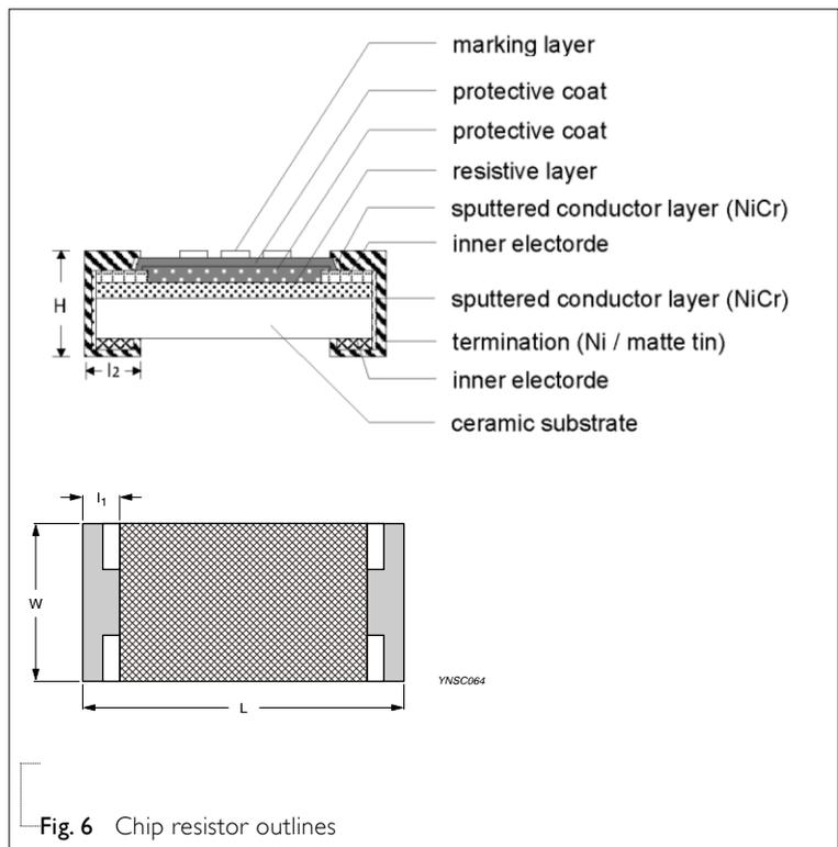
Fig. 6 Chip resistor outlines
