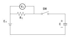
Rc:  $1,000 \Omega$  (0.01 F, 0.022 F, 0.047 F)  $100 \Omega$  (0.10 F, 0.22 F, 0.33 F, 0.47 F)  $10 \Omega$  (1.0 F, 1.4 F, 1.5 F, 2.2 F, 3.3 F, 4.7 F, 5.6 F) However, FS Seres 11 V type and 12 V type  $100 \Omega$  0.47 F, 1.0 F  $10 \Omega$  5.0 F
