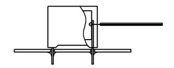
Temperature monitored inside the capacitor.
