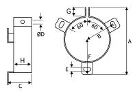
When using mounting clamps, care should be taken not to obscure any safety vent in the can. Delivered without bolts and nuts for mounting. \*PYC clamps are for PEH169 and PEH200 capacitors only. Diameters include platic insulation.
