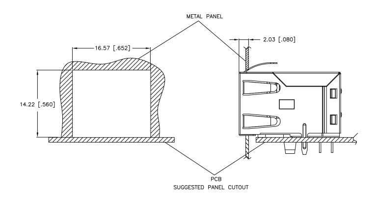
DIMENSIONS ARE IN MILLIMETERS [INCHES] WITH THE FOLLOWING TOLERANCES: [INCHES] ARE FOR REFERENCE ONLY.  $X.XX = \pm 0.10$  [ $\pm .004$ ]
