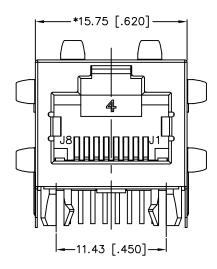
DIMENSIONS ARE IN MILLIMETERS [INCHES] WITH THE FOLLOWING TOLERANCES: [INCHES] ARE FOR REFERENCE ONLY.  $X.XX = \pm 0.10$  [ $\pm .004$ ]
