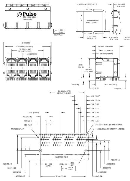
SUGGESTED PC BOARD LAYOUT VIEWED FROM COMPONENT SIDE UNLESS OTHERWISE SPECIFIED DIMENSIONAL TOLERANCE IS ±.002
