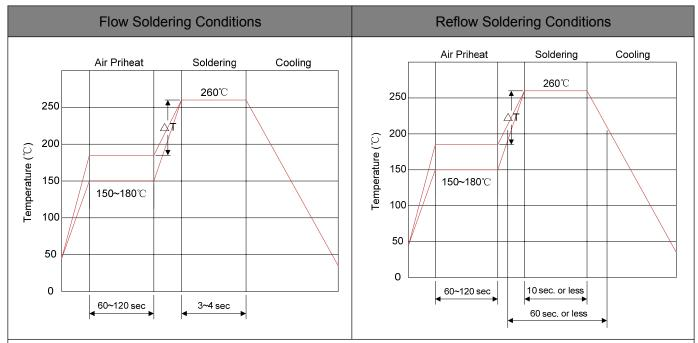
1) Time shown in the above figures is measured from the point when chip surface reaches temperature.
