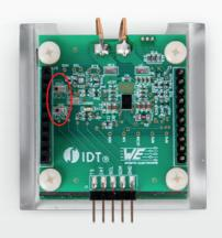
2. Connect your device on those two pads Vout is  $12\,V_{DC}$ . Connect your debug connector to J1 for programming
