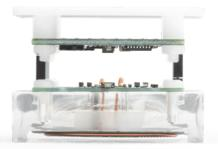
The Receiver System consists of the Receiver and the LED Load Module. Different combinations are available for the users to match their application needs. Please refer to the user manual.
