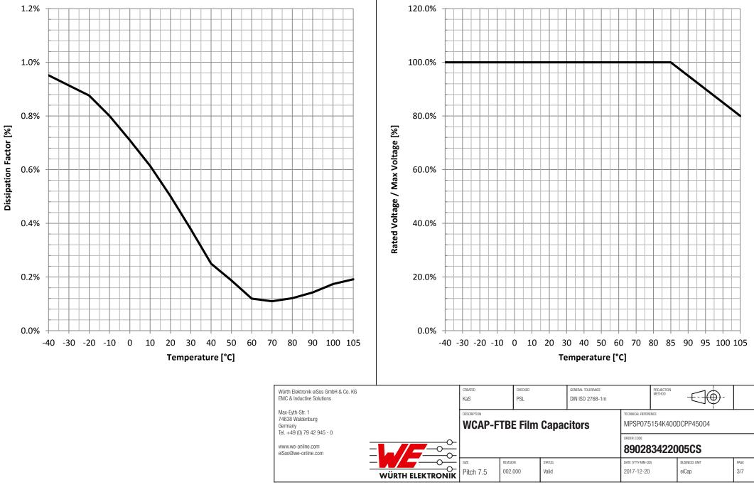
**Rated Voltage vs. Temperature:**
