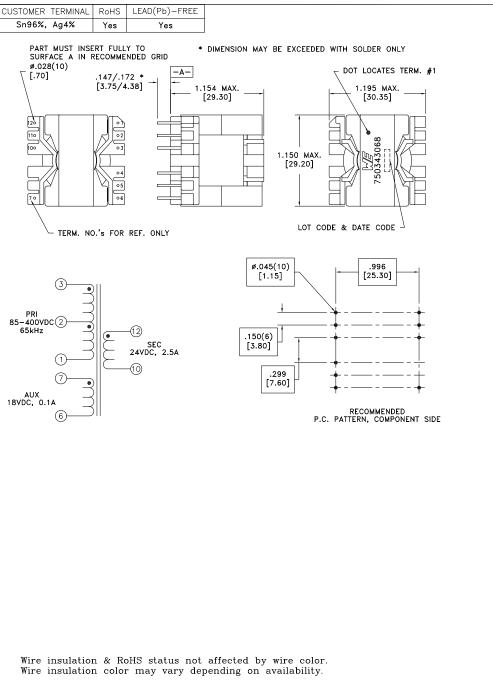
Packaging Specifications DRAWING TITLE PART NO. REV. DATE Tolerances unless otherwise specified: Method: Tray Angles: ±1° Decimals: ±.005 [.13] Footprint: ±.001 [.03] TRANSFORMER PKG-0807 Fractions: ±1/64 750343068 www.we-online.com/midcom This drawing is dual dimensioned. Dimensions CONVENTION PLACEMENT SPECIFICATION SHEET 1 OF 1 eiSos p/n: 750343068 SEE REVISION SHEET FOR REVISION LEVEL 6A 9/16 in brackets are in millimeters.
