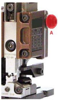
Manually cycle the press by means of a spanner until the terminal is positioned on the anvil. Loosen the nut A and turn the screw clockwise or counter-clockwise to determine the correct position. Then tighten the nut again and make a complete cycle of the press. If the result is not satisfying enough, repeat the operation.
