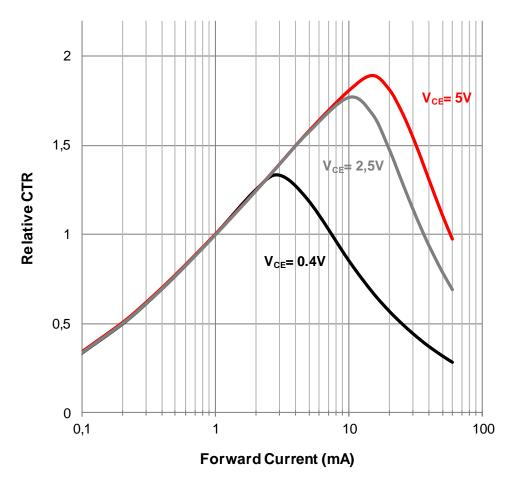
Testcondition: TA=  $25^{\circ}$ C Relative to I<sub>F</sub>= 1mA; TA=  $25^{\circ}$ C
