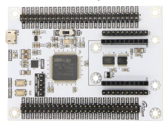
\*COMMENT: P1/P2/P3/P4 have the same function, both arduino compatible with WIZ610MJ, J1,J2 expansion 80 GPIOs (Include analog Peripheral using 12bit ADC).
