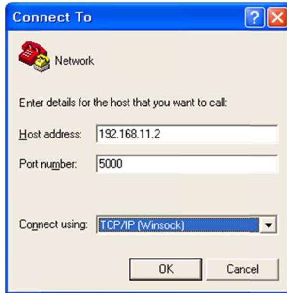
Figure 24. Network Terminal Program configuration
