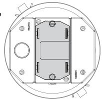
CAUTION: Receptacle supplied with this Poke-Thru is not suitable for direct field wiring. Contact manufacturer for replacement. Field modifications will void UL Listing and Classification. Replacement receptacle is limited to this manufacturers' Catalog No 68REC.
