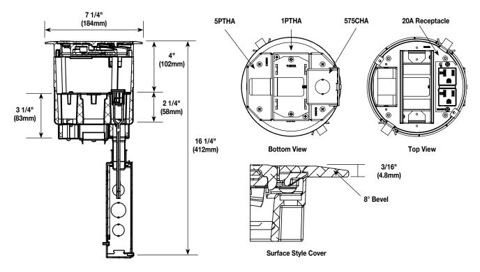
NOTE: For more information on Device Plates and Bottom Feed Plates and on the additional options available, see the Device Plates and Bottom Feed Plates sections found later in this document.
