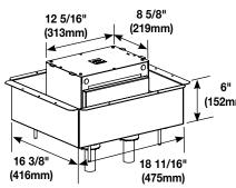
**4- & 5-Gang Fire Classified Floor Box** – Pre-assembled installation ready floor box has been designed to be installed in above grade (second floors and above) concrete floors while maintaining the fire classification of the floor. This box is classified to be used in 2-hour fire rated floors. Designed to accept standard size wall plates. **Box comes complete with all components needed for initial installation.**
