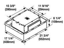
**10-Gang Fire Classified Floor Box** – Pre-assembled installation ready floor box has been designed to be installed in above grade concrete floors while maintaining the fire classification of the floor. This box is classified to be used in 2-hour fire rated floors. Designed to accept standard size wall plates. **Box comes complete** with all components needed for initial installation.
