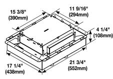
**6-Gang Fire Classified Floor Box** – Pre-assembled installation ready floor box has been designed to be installed in above grade concrete floors while maintaining the fire classification of the floor. This box is classified to be used in the 2-hour fire rated floors. Designed to accept standard size wall plates. **Box comes complete** with all components needed for initial installation.
