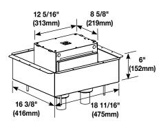
**4- & 5-Gang Fire Classified Floor Box** – Pre-assembled installation ready floor box has been designed to be installed in above grade (second floors and above) concrete floors while maintaining the fire classification of the floor. This box is classified to be used in 1-, 1 1/2-, 2- or 3-hour fire rated floors. Designed to accept standard size wall plates. Box comes complete with all components needed for initial installation.
