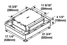
**6-Gang Fire Classified Floor Box** – Pre-assembled installation ready floor box has been designed to be installed in above grade concrete floors while maintaining the fire classification of the floor. This box is classified to be used in 1-, 1 1/2-, 2-, or 3-hour fire rated floors. Designed to accept standard size wall plates. **Box comes complete with all components needed for initial installation.**
