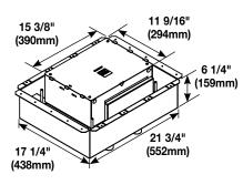
**10-Gang Fire Classified Floor Box** – Pre-assembled installation ready floor box has been designed to be installed in above grade concrete floors while maintaining the fire classification of the floor. This box is classified to be used in 1-, 1 1/2-, 2-, or 3-hour fire rated floors. Designed to accept standard size wall plates. **Box comes complete with all components needed for initiainstallation.**
