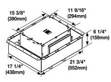
**8-Gang Fire Classified Floor Box** – Pre-assembled installation ready floor box has been designed to be installed in above grade concrete floors while maintaining the fire classification of the floor. This box is classified to be used in 2-hour fire rated floors. Designed to accept standard size wall plates. **Box comes complete with all components needed for initial installation.**
