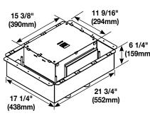
**8-Gang Fire Classified Floor Box** – Pre-assembled installation ready floor box has been designed to be installed in above grade concrete floors while maintaining the fire classification of the floor. This box is classified to be used in 1-, 1 1/2-, 2-, or 3-hour fire rated floors. Designed to accept standard size wall plates. **Box comes complete with all components needed for initial installation.**
