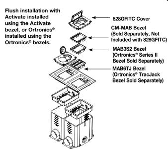
Recessed installation with Activate installed directly into the 880MPA Adjusting Ring. Ortronics® inserts cannot be inserted directly into 880MPA, see below for Ortronics® solution.
