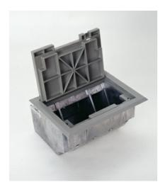
The AF1 Raised Floor and Stage Floor Box provides three separate compartments that accommodate a combination of power, communication and audio/video devices. This combination is accomplished with the built-in service dividers. These dividers are arranged in a single-double, single-gang configuration. Die-cast aluminum housing provides added strength and reliability. Polycarbonate
