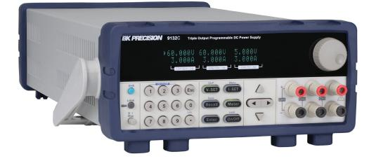
The 913OC Series triple output linear programmable DC power supplies feature isolated outputs that can be adjusted independently or combined in series or parallel to output higher voltage or current. Additionally, these supplies can operate in tracking mode with user-configurable ratios between channels.
