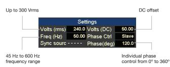
Set voltage, frequency, and phase directly from the front panel on each AC source.
