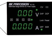
The 9110 is a new type of power supply. Unlike conventional power supplies with fixed output ratings, the 9110 automatically recalculates voltage/current limits for each setting. The 9110 provides 100 W output power in any Volt/Amp combination within the rated voltage (60 V) and current (5 A) limits. By providing greatly expanded choices of maximum power Volt/Amp combinations, users can cut down on the number of power supplies required and free up valuable bench space.
