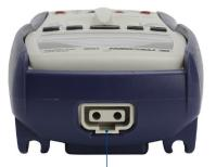
Optical isolated USB interface for PC connectivity
