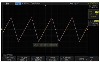
A powerful 25 MHz function/arbitrary waveform generator comes standard in the 2540C Series. Use complimentary software to generate waveforms and load up to 4 arbitrary waveforms into the instrument. Built-in functions are sine, square, ramp, pulse, DC, noise, cardiac, Gaussian pulse, and exponential rise/fall.
