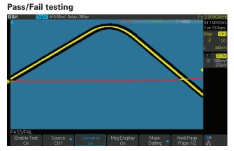
Generate a mask based on user defined parameters to identify pass/fail test results. Useful in long term signal monitoring or automated production line testing applications.
