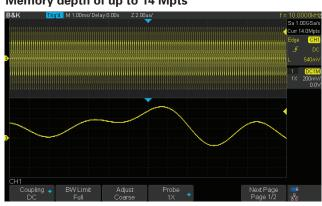
Capture longer time periods at higher resolution with a maximum memory depth of I4 Mpts. Enable zoom feature to display specific events in more detail.
