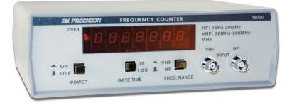
The 1803D is a value-priced frequency counter offering users a simple and accurate frequency measurement.
