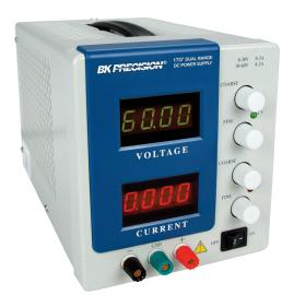
B&K Precision's model 1737 is a general purpose dual range DC power source. This power supply can output higher voltage at a lower current range or higher current at a lower voltage range. Two 4-digit LED displays continuously monitor the output voltage and current. The power supply can be operated locally from the front panel or remotely through the RS-232 interface.
