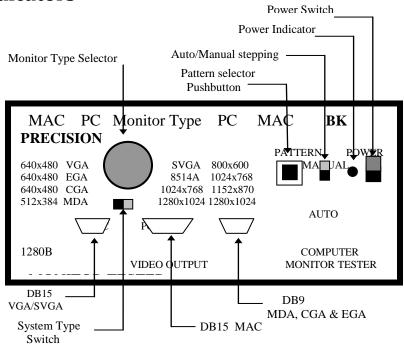
**Power** -- Slide switch for power on or off.
