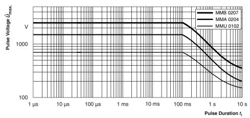
Maximum pulse voltage, single and continuous pulses; applicable if  $\hat{P} \le \hat{P}_{\text{max}}$ ; for permissible resistance change  $\pm$  (0.5 % R + 0.01  $\Omega$ )
