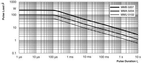
Maximum pulse load, single pulse; applicable if  $\vec{P}$   $\rightarrow$  0 and n  $\leq$  1000 and  $\hat{U} \leq \hat{U}_{\text{max}}$ ; for permissible resistance change  $\pm$  (0.5 % R + 0.01  $\Omega$ )
