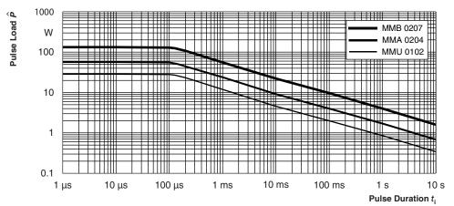
Maximum pulse load, continuous pulse; applicable if  $\bar{P} \leq P$  (9<sub>amb</sub>) and  $\hat{U} \leq \hat{U}_{\text{max}}$ ; for permissible resistance change  $\pm$  (0.5 % R + 0.01  $\Omega$ )
