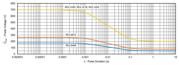
Maximum pulse voltage, single and continuous pulses; applicable if  $\ddot{P} \leq \dot{P}_{max}$ ; for permissible resistance change equivalent to 8000 h operation
