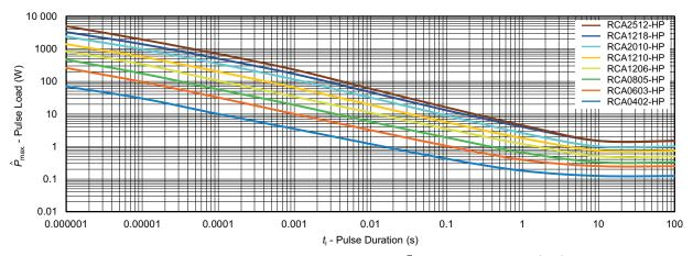
Maximum pulse load, single pulse; applicable if  $\bar{P} \to 0$  and n < 1000 and  $\hat{U} \le \hat{U}_{max}$ ; for permissible resistance change equivalent to 8000 h operation
