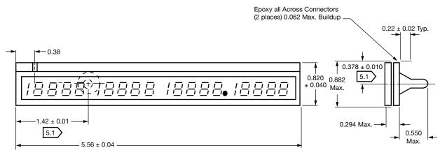
5.1 Fill tube is concentric with hole within  $\pm$  0.060 vertically and + 0.060/- 0.030 horizontally.
