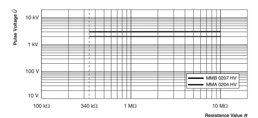
Pulse load rating in accordance with IEC 60 115-1, 4.27; 1.2 µs/50 µs; 5 pulses at 12 s intervals; for permissible resistance change (0.5 % R + 0.05  $\Omega$ )
