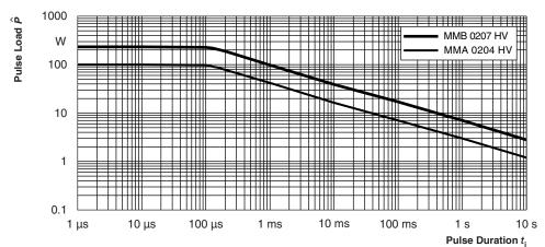
Maximum pulse load, single pulse; applicable if  $\bar{P}$  → 0 and n ≤ 1000 and  $\hat{U}$  ≤  $\hat{U}_{max}$ ; for permissible resistance change ± (0.5 % R + 0.01  $\Omega$ )
