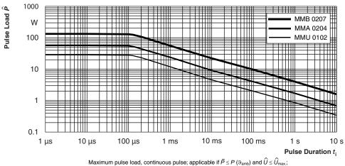
Maximum pulse load, continuous pulse; applicable if  $P \le P$  ( $9_{amb}$ ) and  $U \le U_m$  for permissible resistance change ± (0.5 % R + 0.01  $\Omega$ )
