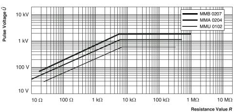
Pulse load rating in accordance with IEC 60115-1, 4.27; 10 µs/700 µs; 10 pulses at 1 minute intervals; for permissible resistance change  $\pm$  (0.5 % R + 0.05  $\Omega$ )
