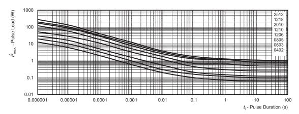
Maximum pulse load, continuous pulses; applicable if  $\overline{P} \le P(\mathcal{G}_{amb})$  and  $\hat{U} = \hat{U}_{max}$ ; for permissible resistance change equivalent to 8000 h operation
