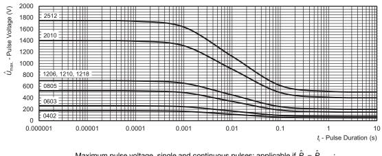
Maximum pulse voltage, single and continuous pulses; applicable if  $\hat{P} = \hat{P}_{max}$ ; for permissible resistance change equivalent to 8000 h operation
