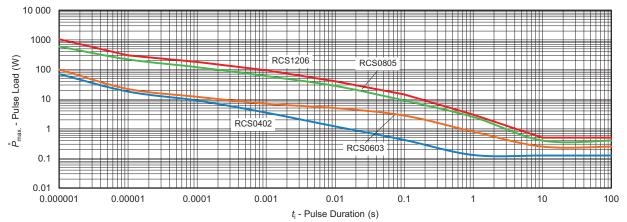
Maximum pulse load, single pulse; applicable if  $\overline{P} \to 0$  and n < 1000 and  $\hat{U} = \hat{U}_{\text{max}}$ ; for permissible resistance change equivalent to 8000 h operation
