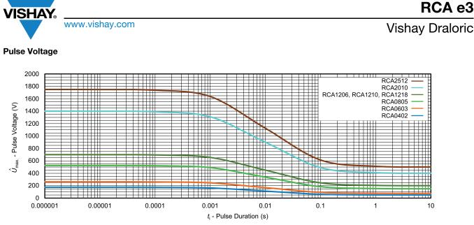
Maximum pulse voltage, single and continuous pulses; applicable if  $\hat{P} = \hat{P}_{max}$ ; for permissible resistance change equivalent to 8000 h operation
