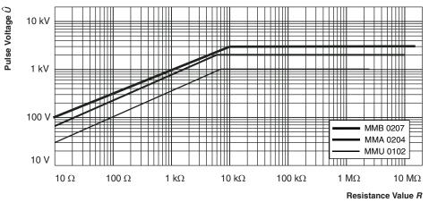
Pulse load rating in accordance with IEC 60 115-1, 4.27; 1.2 µs / 50 µs; 5 pulses at 12 s intervals; for permissible resistance change  $\pm$  (0.5 % R + 0.05  $\Omega$ )
