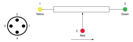
Direction of wiper displacement with shaft extended
