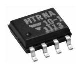
HTRN series resistor networks feature four isolated resistors with standard 50 mil pitch lead spacing. HTRN is ideal to be used in oil/gas exploration industry, automotive under the hood applications, and aerospace engine control high temperature applications. The networks feature close TCR tracking and tight ratio tolerance and are ideally suited for unity gain operational amplifier circuitry. The standard resistance offering listed are available for immediate delivery.
