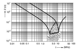
Measurement with lead length 6 mm.
